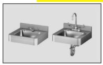
Price Includes: 16 gage 304 Stainless Steel Rectangular Lavy, 20" wide x 18" Deep with 14-1/2" x 12" x 6" integral bowl, 3" integral backsplash, sleeves to accommodate carrier by others and three holes (1-5/16" Dia.) punched on 4" center to accommodate valve by others.
