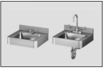
Price Includes: 16 gage 304 Stainless Steel Rectangular Lavy, 18" wide x 18" Deep with 14-1/2" x 12" x 6" integral bowl, 3" integral backsplash and three holes (1-5/16" Dia.) punched on 4" center to accommodate valve by others.
