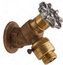
FIG. 5670-H HOSE VALVE BENT NOSE WITH FLANGE W/ASSE 1011 VACUUM BREAKER
